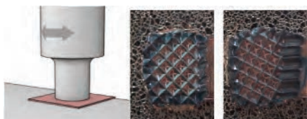
Minimum scooting observed with torsional welding versus longitudinal welding on a same application
