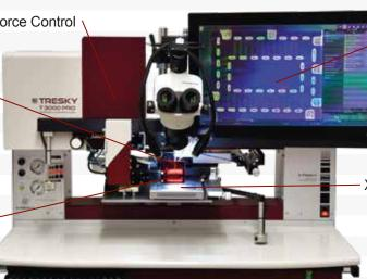
Interface for all bonding parameter, temperature profile and video imaging of Beam Splitter Optics, Process Inspection Camera
